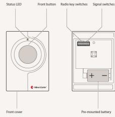
Look at the back of the main case and carefully drill a hole no more than 4mm diameter through each of the marked cut-outs, top right hand and lower left hand edges. Select two suitable screws (ask us to send them!) and attach the push button to the doorframe at a suitable height.
